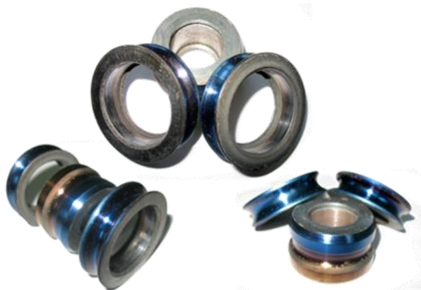
Experimental samples of ion-plasma- modified working surfaces of equipment used for drawing wire/
