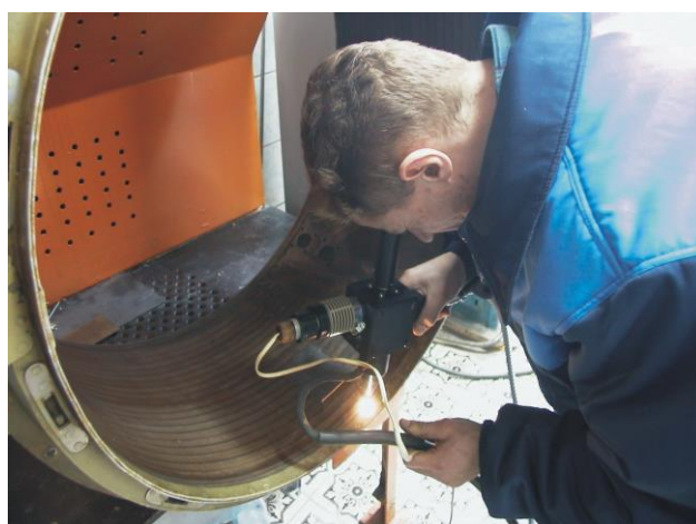
Processing of a large machine part at a remove from laser installation using a fiber-optic system. /
