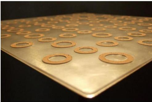
From a practical point of view, the developed metasurfaces can be used for the purpose of shielding electronic devices. At the same time, metasurfaces absorb radiation of a given range exclusively selectively, allowing waves of other frequencies outside this range to be reflected from the structure in the opposite direction practically without signal attenuation..
